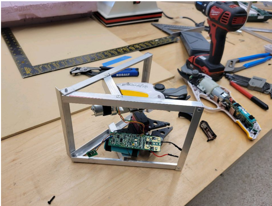
Figure 7. Cutting mechanism showing housing modification.
